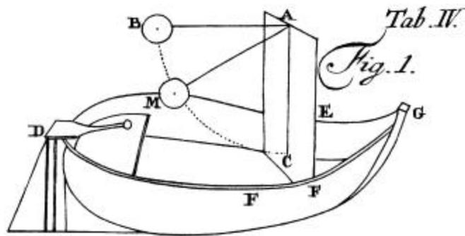
Bernoulli proposed to erect a wall near the bow of the ship and to suspend a heavy weight from the top of the wall at the point marked A. He would lift the ball to the point B and let it drop. It would swing through M, strike the wall at C, and propel the boat forward. At the same time, he hoped, the ball would bounce back to B, from which it would fall again and propel the boat forward again. Obviously, Bernoulli never actually tested his design. It would have been a rough ride.
