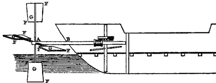
Euler's final idea is almost futuristic. His idea, pictured below, is to try to harness the motion of waves to move a ship. He proposes to put a trough, AEFB just above water level in the stern of the ship.
