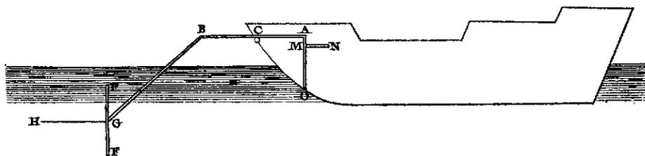
Here, we have a vertical surface, FF, attached to a bent support ACBG and suspended from the front of the boat. Workers inside the boat pull the system along the path MN, then lift it out of the water, push it forward and lower it back in to the water. It works kind of like a hoe. Euler decides it isn't really a very good idea.
