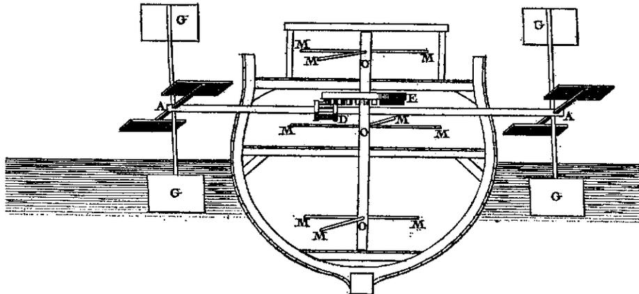
Euler's fourth idea also would not prove useful until the 19<sup>th</sup> Century. Shown below, he proposed extending a kind of fan in front of the ship, then turning it with the same kind of mechanism that he had used for the paddle wheel. This idea was patented in 1838 by the Swedish inventor John Ericsson. Ericsson had in mind that the propeller would be turned by a steam engine.
